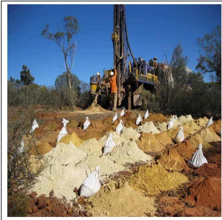
Figure 2: RAB drilling, September quarter 2010
